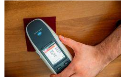
PORTABLE SPECTROPHOTOMETER FOR USE IN THE TANNERY
